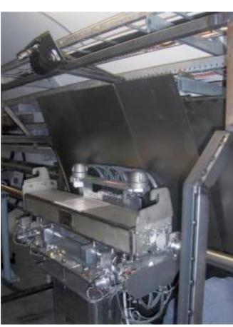
Magnetic screens installed to shield the collimators (A. Masi)
